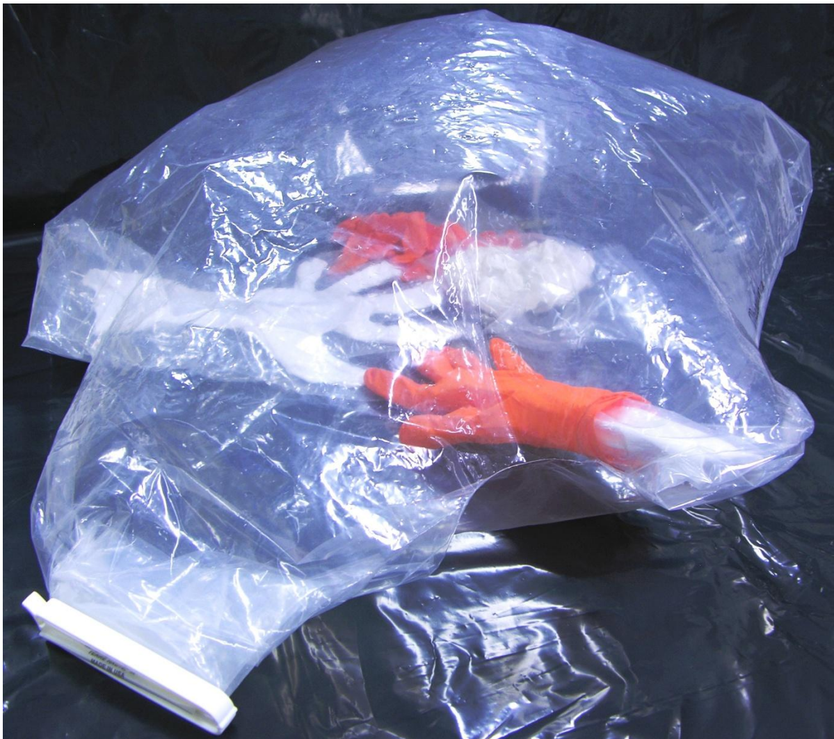
Figure 1. Photograph of glove-bag used as part of the sample preparation to minimise chances of cross contamination
