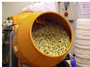
Figure 2 Bulk Sample Mixing using a Cement Mixer (courtesy Kent Scientific Services)
