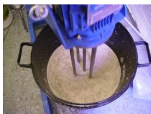
Figure 3 Slurrying with Water (courtesy Kent Scientific Services)
